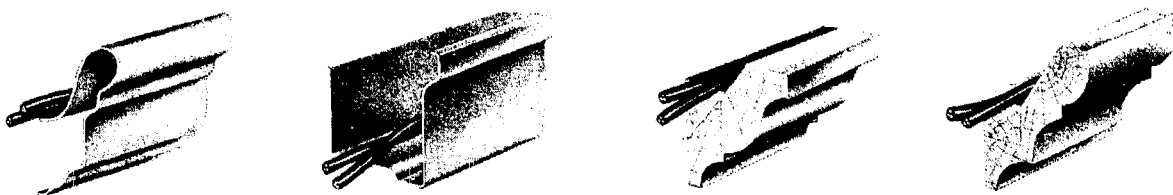
Fig. 10 – Wiring in Picture Moldings
