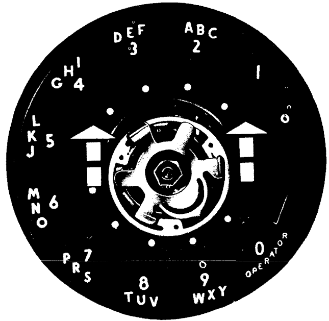
Fig. 8 — Lock Ring in Extreme Forward Position for Removal
