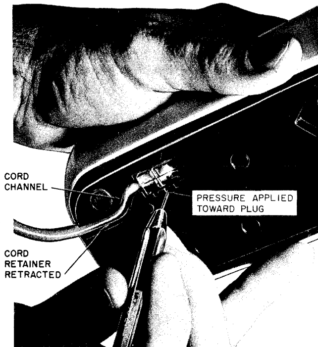
Fig. 12—Removing Mounting Cord From AD1 telephone Base
